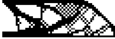
Figure A1. Checkerboard phenomenon in topology optimization using the SIMP model.
