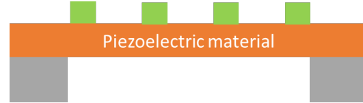
Figure 7. XBAR resonator structure
