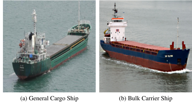
Figure 1: An example of a general cargo ship and a bulk carrier ship.
