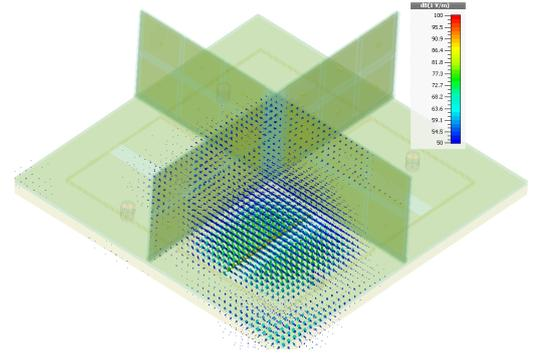
Fig.4. The simulated E-field distribution (excited by Antenna 1 at 2.42 GHz)
