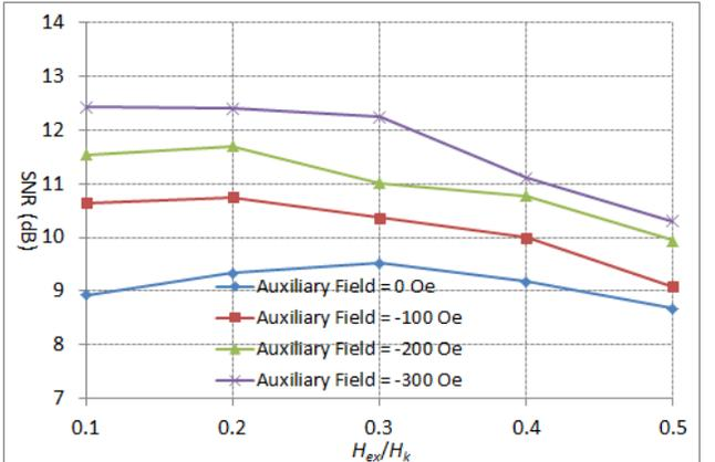
Fig. 7. SNR of the HAMR recording while the  $H_{ex}/H_k$  is set from 0.1 to 0.5 and  $\sigma_{ez} = 3^\circ$ .
