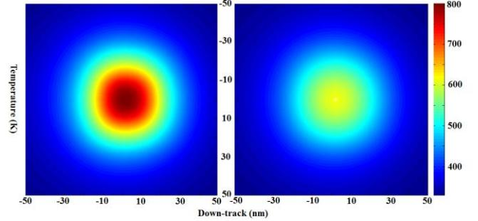
Fig. 3. Thermal spot distribution (left: top layer; right: bottom layer).
