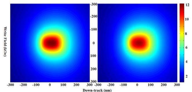
Fig. 1. Write field distribution (left: top layer; right: bottom layer).
