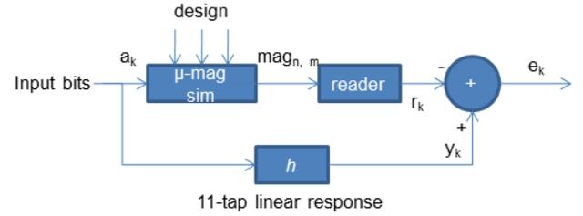
Fig. 4. Block Diagram showing components used in the SNR calculation. cross-correlation matrix between  $a_k$  and  $r_k$ . In the context of Figure 4, the SNR is then obtained as the ratio of the powers:
