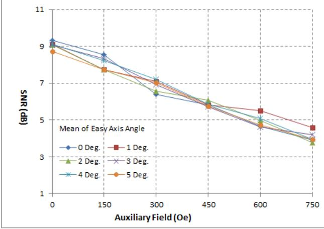
Fig.8. SNR of the HAMR recording while an auxiliary field in the down-track direction is applied ( $H_{ex}/H_k = 0.1$ ).
