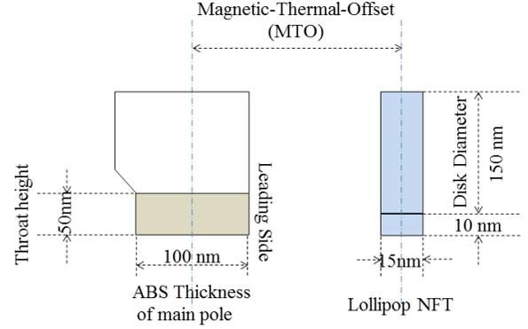
Fig. 2. The model of the relevant parts of the write head and the NFT and their locations.
