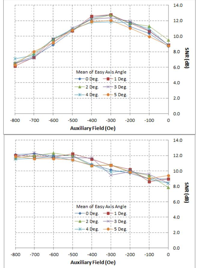
Fig. 6. SNR of the HAMR recording with  $H_{aux}$  of 0 Oe to  $-800$  Oe when  $H_{ex}/H_k = 0.1$  (top), 0.5 (bottom) respectively.
