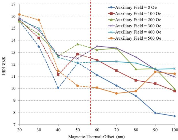
Fig.9. SNR of the HAMR recording while an auxiliary field in the down-track direction is applied ( $H_{ex}/H_k = 0.1$ ).
