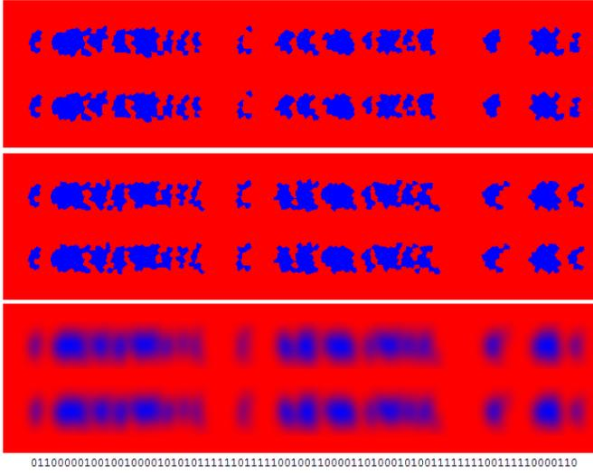
Fig. 5. A partial view of the magnetization profile of the HAMR recording with bit pattern and 2D read-back signal after convolution:  $H_{ex}/H_k = 0.3$ ,  $\sigma_{ez} = 3^\circ$  (Top:  $H_{aux} = 0$  Oe; Middle:  $H_{aux} = -600$  Oe; Bottom: read-back signal after convolution with the RHS functions while  $H_{aux} = -600$  Oe; ).
