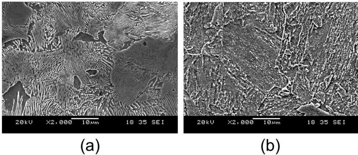
**Fig. 1** As-received microstructures of **a** AISI 1055 steel showing ferrite and pearlite, and **b** 50CrMo4 steel showing elongated carbides in ferritic matrix
