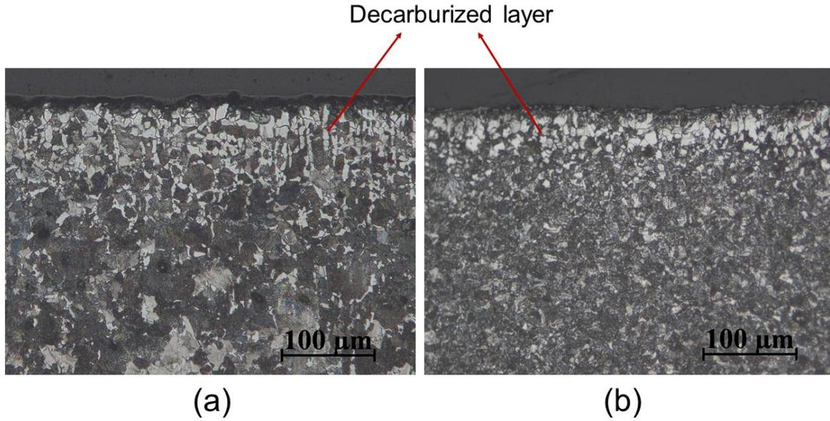
**Fig. 2** Decarburized surface layers of **a** AISI 1055 steel, and **b** 50CrMo4 steel after the heat treatment in furnace
