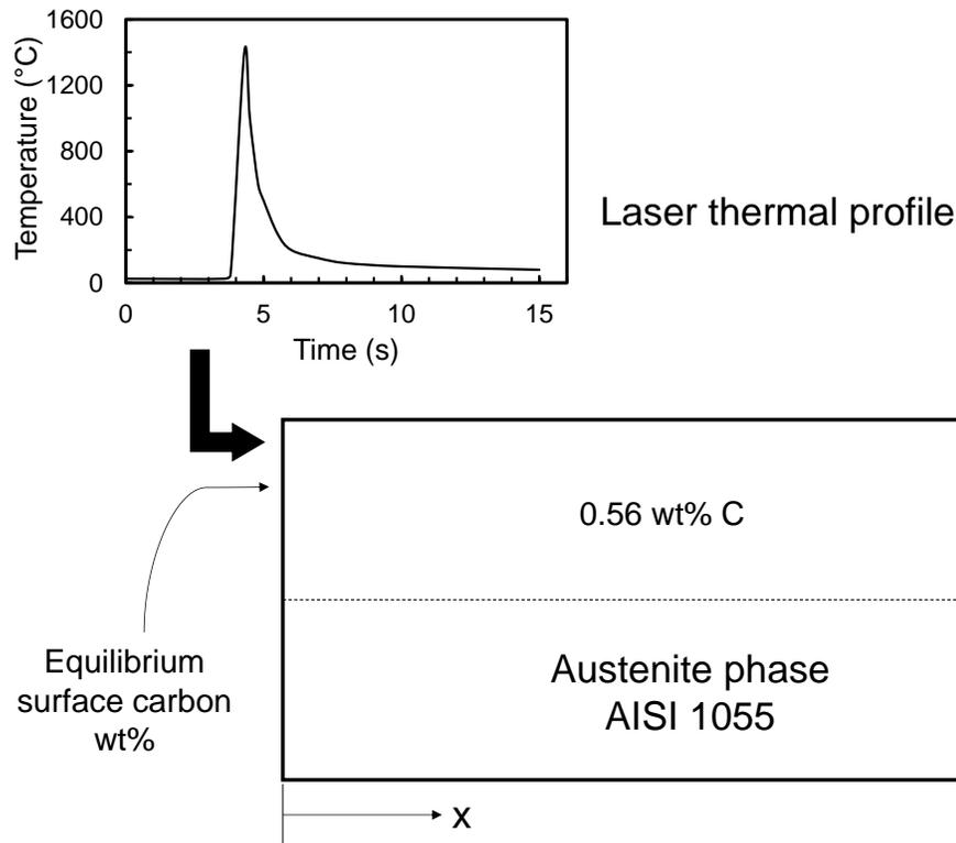
**Fig. 6** Geometric scheme for modelling of decarburization during laser processing
