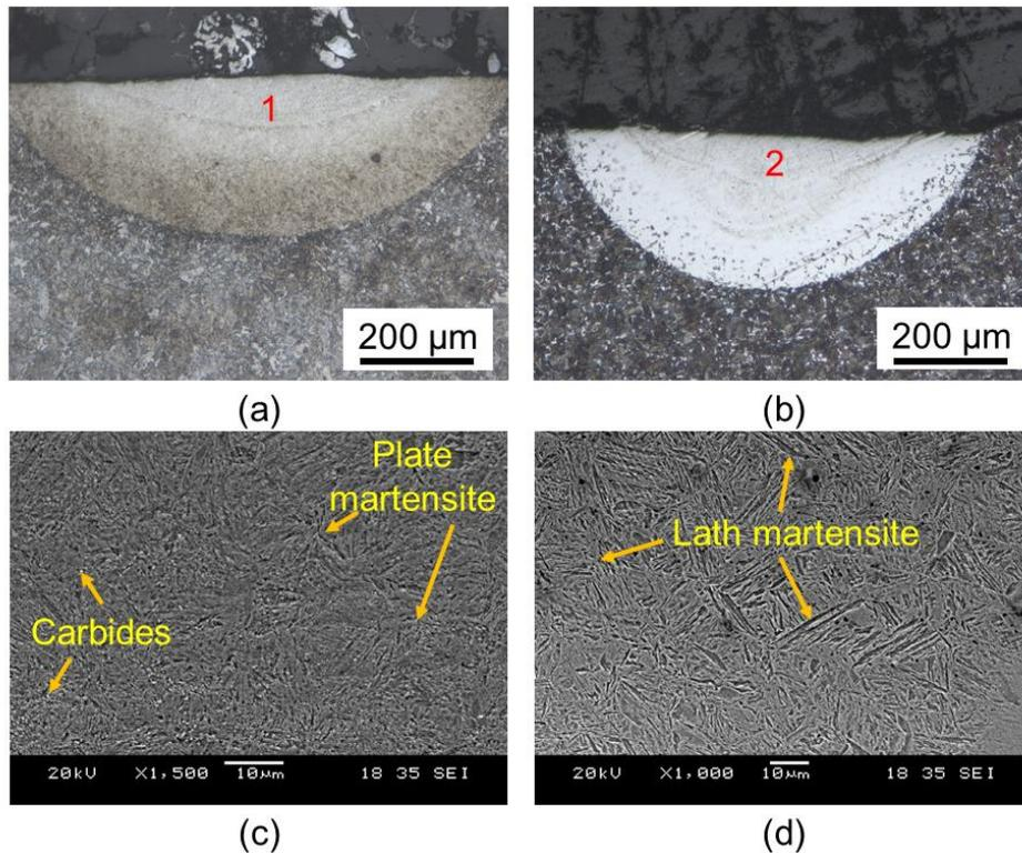
**Fig. 4** Micrographs showing laser treated region of 50CrMo4 steel (a,c) and AISI 1055 steel (b,d) – **a,b** OM images showing overall laser affected region, and **c,d** SEM images showing higher magnification of region marked as “1” and “2” in a and b respectively
