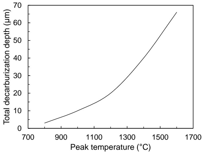
**Fig. 8** Variation of decarburization depth with peak temperature during laser surface processing
