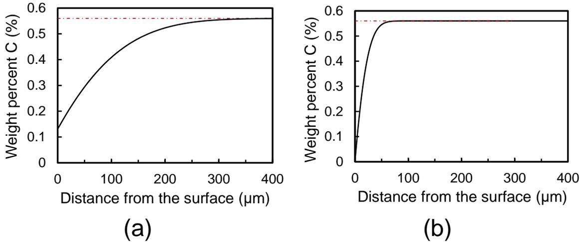
**Fig. 7** Modelling results showing loss of carbon from the surface for **a** furnace heat treatment, and **b** laser surface treatment
