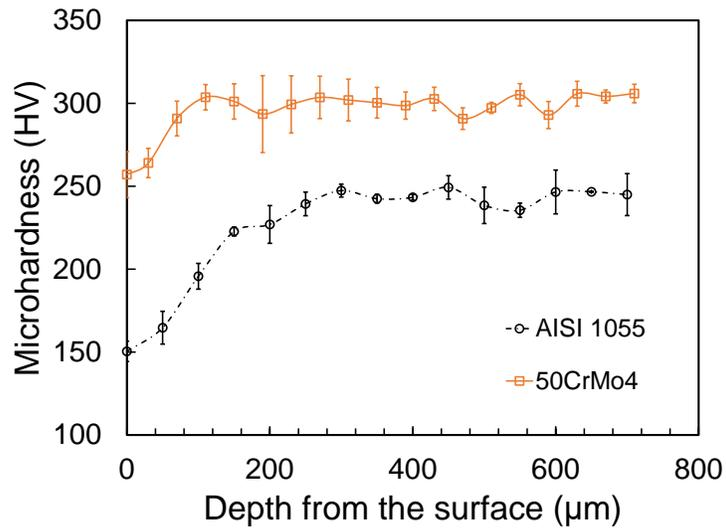
**Fig. 3** Vickers microhardness profile showing decrease in surface hardness after the furnace heat treatment
