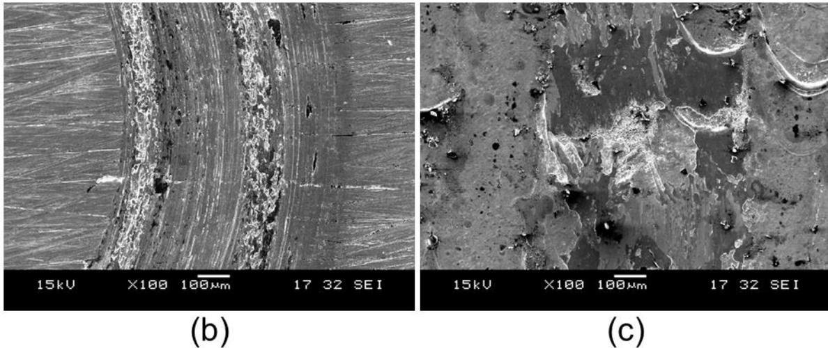
**Fig. 9** Comparison of wear resistance of as-received and laser treated surfaces – **a** plot of mass loss against time, **b** wear morphology of as-received surface, and **c** wear morphology of laser treated surface
