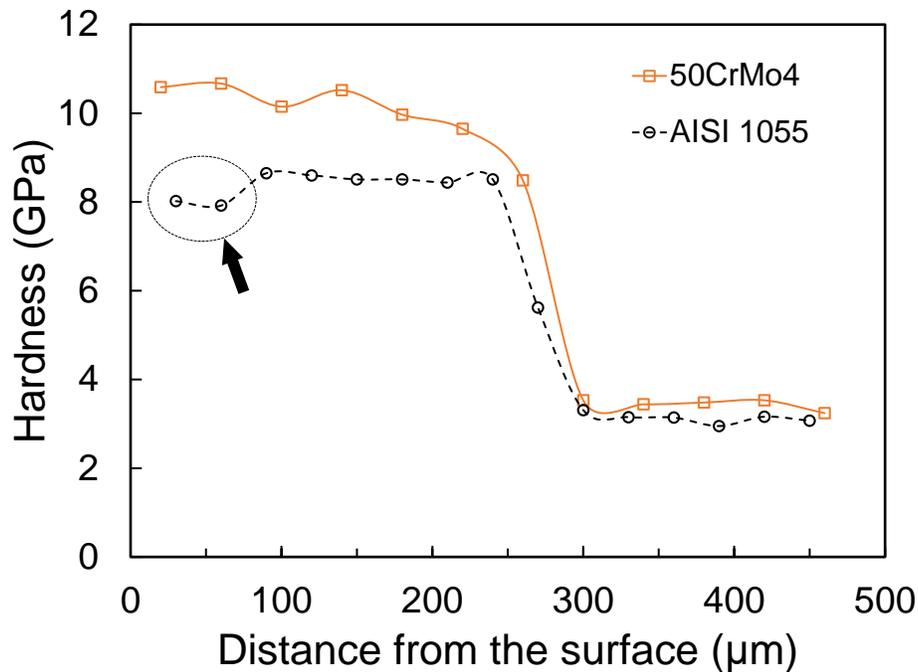
**Fig. 5** Berkovich hardness profile after laser processing showing hardened surfaces for both steels but slightly lower hardness values (arrowed) for the top 100  $\mu\text{m}$  surface layer of AISI 1055 steel
