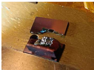
Figure 18: Optical image of the sample after shear test
