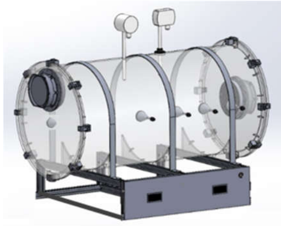
Fig. 1. A CAD drawing for the droplet test chamber. The droplet generator is connected to the left side of the chamber for ejection of droplets into the chamber. Clean air is blown from left side to flush the chamber before each measurement experiment.
