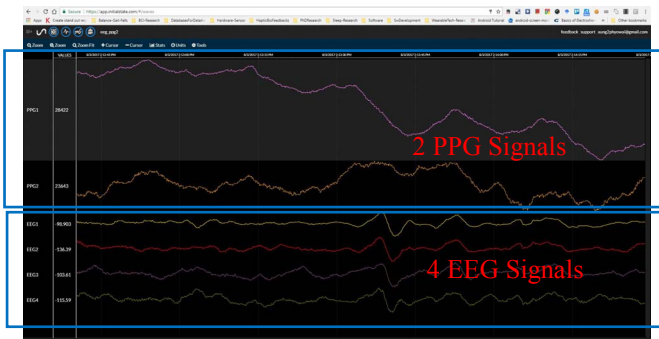
Fig. 8. Real-time streaming and visualization of EEG + PPG signals from iMESH headwear over cloud using library from Initial State Technologies
