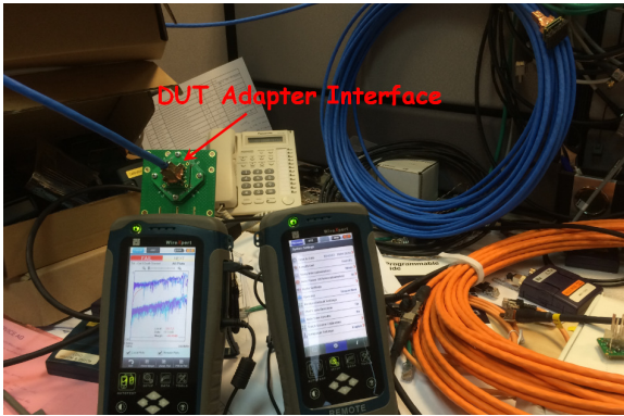
(a) Field tester measurements done with a DUT adapter
