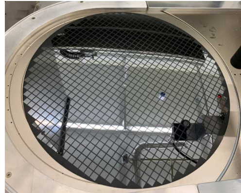
Figure 8: Wafer not stopping at chuck's centre
