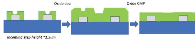
Fig.5 Dielectric with planarization process flow
