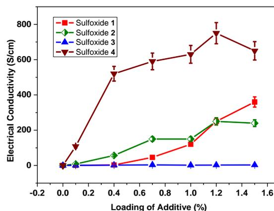
**Figure 3.** Electrical conductivity for the PEDOT:PSS films doped with the respective sulfoxides.
