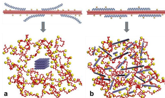
**Figure 2.** A proposed molecular mechanism for thermoelectric enhancement by using the sulfoxide derivatives. a) The additives (yellow) that have strong interaction with the PSS phase (red) lead to the PEDOT:PSS phase separation and PEDOT (blue) aggregation via charge screening, b) Additives that mix with both PSS and PEDOT cannot enhance thermoelectric properties.
