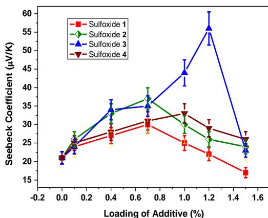
**Figure 4.** Seebeck coefficient of PEDOT: PSS films doped with 4 additives.
