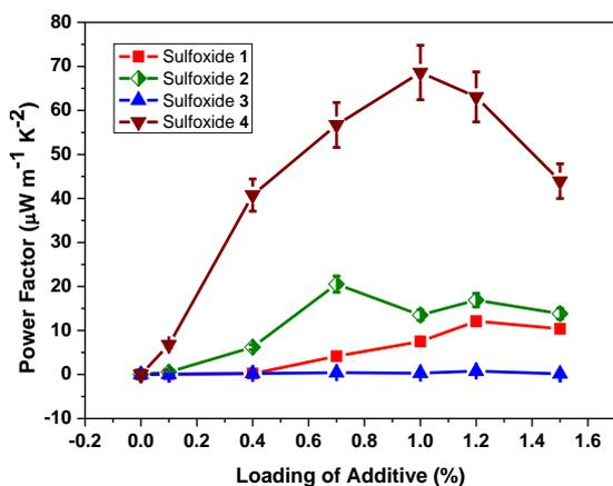
**Figure 5.** Power factor of PEDOT: PSS films doped with 4 additives.
