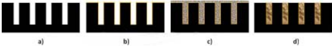
Fig. 1. Conventional TSV integration procedure. (a) Si etch. (b) Dielectric/Cu BS deposition. (c) TSV Cu filling. (d) Annealing/CMP.
