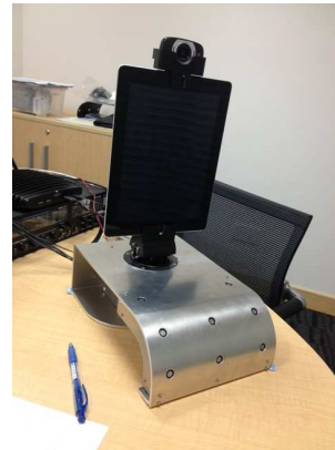
Figure 2: The prototype of the pan-tilt robotic base with a smart tablet.
