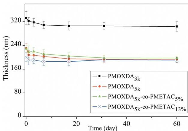
**FIGURE 3** Coating thickness versus time of the different surfaces (composition and explanation of symbols are shown in the inset) as measured by surface profiler. Error bars correspond to standard deviations.
