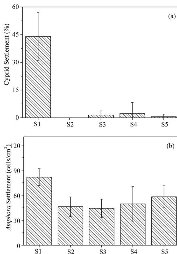
**FIGURE 5** (a) Cyprids of *Amphibalanus amphitrite* and (b) *Amphora coffeaeformis* settlement on different surface. Error bars correspond to the standard deviations. S1:Si; S2:PMOXDA<sub>3k</sub>; S3:PMOXDA<sub>5k</sub>; S4:PMOXDA<sub>5k</sub>-co-PMETAC<sub>5%</sub>; S5: PMOXDA<sub>5k</sub>-co-PMETAC<sub>13%</sub>.
