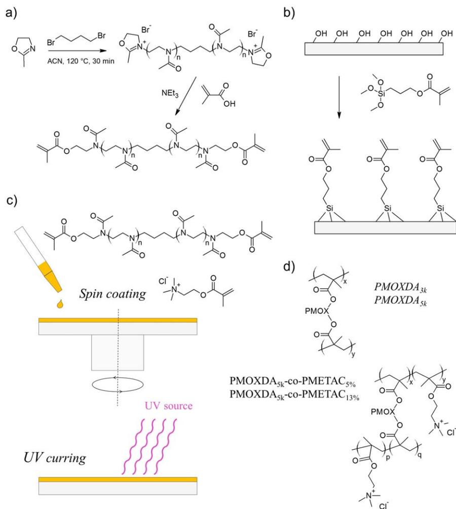
**SCHEME 1** (a) Living cationic ROP of 2-methyl-2-oxazoline initiated by 1,4-dibromobutane and end capping with methacrylic acid; (b) Silane treatment of Si wafer; (c) Film fabrication by spin coating and UV crosslinking; (d) Chemical structure of the crosslinked films.
