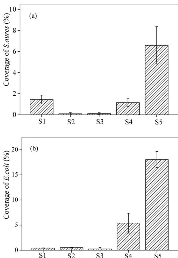
**FIGURE 4** Bacteria coverage on different coating surfaces of (a) *S. aureus*, (b) *E. coli* adhesion assays. Error bars correspond to the standard deviations. S1:Si; S2:PMOXDA<sub>3k</sub>; S3:PMOXDA<sub>5k</sub>; S4:PMOXDA<sub>5k</sub>-co-PMETAC<sub>5%</sub>; S5: PMOXDA<sub>5k</sub>-co-PMETAC<sub>13%</sub>.
