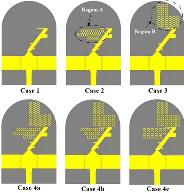
Fig. 3. Configuration of the top layer of the antenna prototypes with different distribution of the MTM inclusions.
