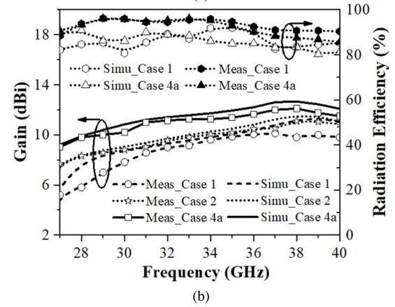
Fig. 7. Measured and simulated (a)  $|S_{11}|$  of the CMPLPDA antennas for Cases 1, 2, and 4a, and (b) gain and efficiency of the CMPLPDA antennas for Cases 1 and 4a.
