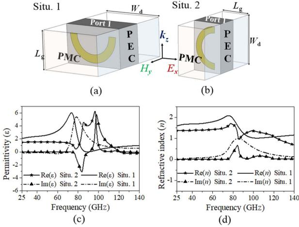
Fig. 1. Two simplified situations for the wave propagating in the  $z$ -direction and the  $E$ -field parallel to the semiring patch. (a) Situ. 1. (b) Situ. 2. (c) Retrieved relative permittivity for both Situ. 1 and Situ. 2. (d) Retrieved refractive index for both Situ. 1 and Situ. 2.
