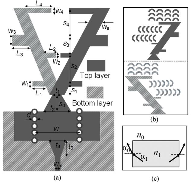
Fig. 2. (a) Geometry of the CMPLPDA antenna. (b) Top and bottom surfaces of the CMPLPDA antenna without SIW. (c) Theoretical model of the proposed nonresonant MTM.
