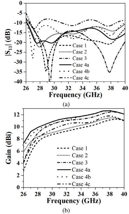
Fig. 4. Simulated (a)  $|S_{11}|$  and (b) gains of the four different cases of the PLPDA antenna.
