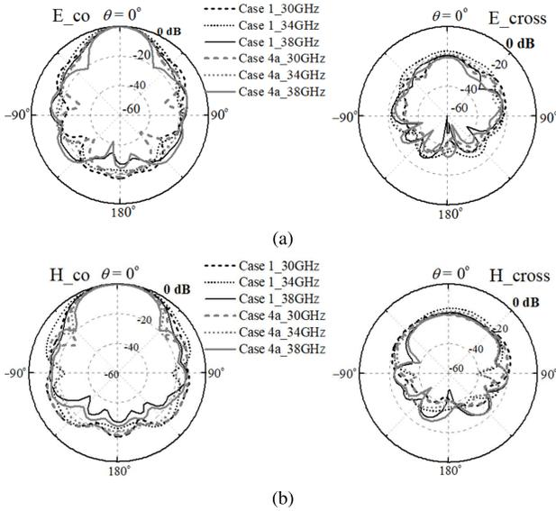
Fig. 8. Normalized copol/cross-pol patterns of the CMPLPDA antennas with/without MTM. (a) E-plane. (b) H-plane. (E/H\_co: copolarization in E-/H-planes, E/H\_cross: cross polarization in E-/H-planes.)
