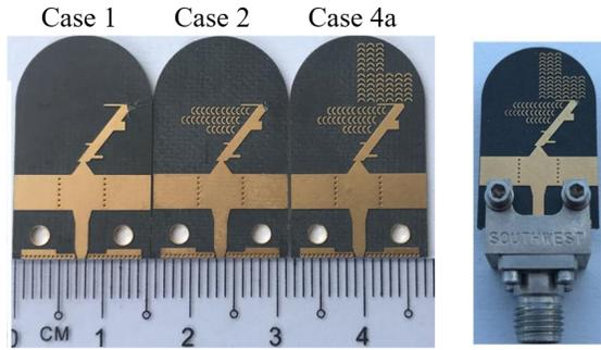
Fig. 6. Top view of the photographs of the CMPLPDA antennas for Cases 1, 2, and 4a, and the CMPLPDA antenna for Case 4a with the end-launcher.
