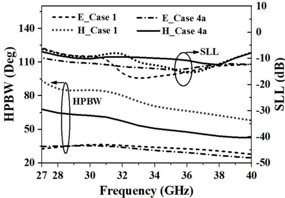
Fig. 9. Comparisons of the HPBW and SLL for the PLPDA antennas for Cases 1 and 4a.
