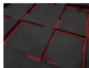
Fig. 20. Close-range hybrid weld (corner weld, end weld, T shape)
