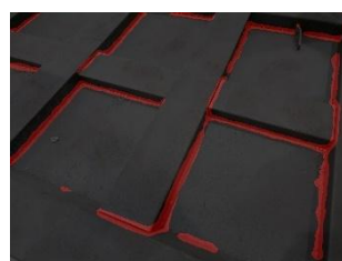
Fig. 20. Close-range hybrid weld (corner weld, end weld, T shape)
