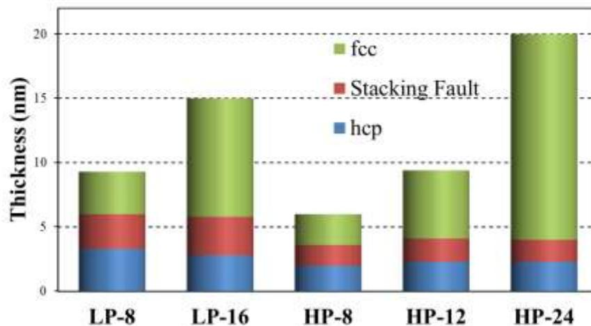
**FIG. 6.** (Color online) Summary of fcc, SF and hcp thickness measured in HRTEM for samples deposited at low pressure (LP) and high pressure (HP). The value after LP/HP is the targeted CoPt thickness.
