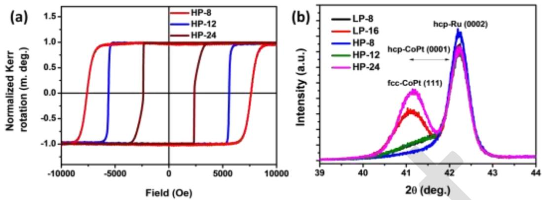
**FIG. 1.** (Color online) (a) MOKE hysteresis loops of CoPt thin films of different thickness deposited at 96 mTorr. (b) XRD patterns of CoPt samples deposited at various pressures and with various thickness. The number after LP or HP indicates the targeted thickness of CoPt layer in nm.
