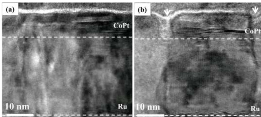
**FIG. 7.** Low magnification TEM images of samples deposited at (a) low and (b) high Ar pressures, respectively.
