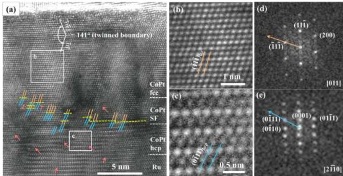
**FIG. 4.** (Color online) (a) HRTEM image of the CoPt from Sample LP-16 where the layer can be divided into CoPt<sub>fcc</sub>, SF and CoPt<sub>hcp</sub> regions. (b, c) The corresponding enlarged HRTEM images of Regions b and c. (d, e) Corresponding FFTs of Regions b and c.
