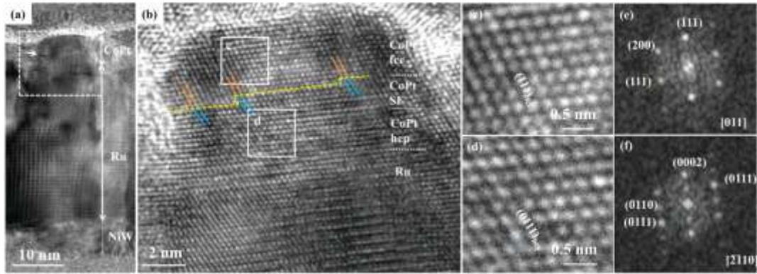
**FIG. 5.** (Color online) (a) HRTEM image of the epitaxial grown CoPt/Ru/NiW layers of Sample HP-8. (b) Enlarged HRTEM image of the CoPt where the layer can be divided into  $\text{CoPt}_{\text{fcc}}$ , SF and  $\text{CoPt}_{\text{hcp}}$  regions. (c, d) Corresponding enlarged HRTEM images of Regions c and d, and (e, f) corresponding FFTs of Regions c and d in (a).
