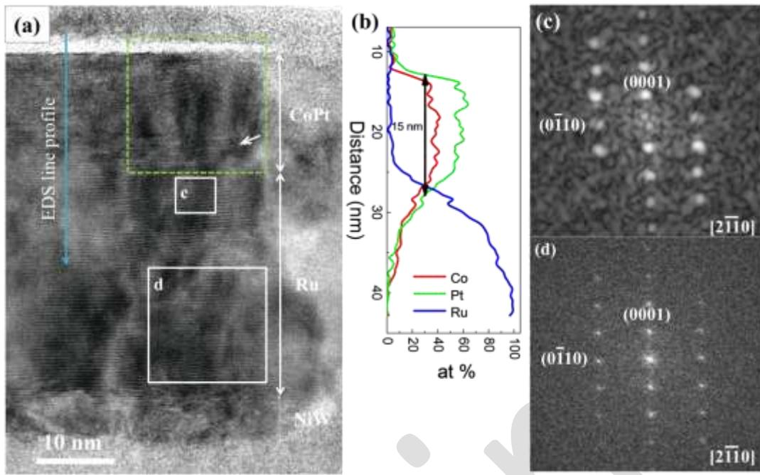
**FIG. 3.** (Color online) (a) HRTEM image of the epitaxially grown CoPt/Ru/NiW layers of Sample LP-16. (b) The EDS line profile of sample corresponding to (a). (c) and (d) Corresponding FFTs of Regions c and d in (a).
