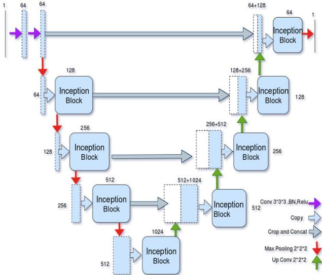
Fig 3. Block Diagram of Inception U-Net.
