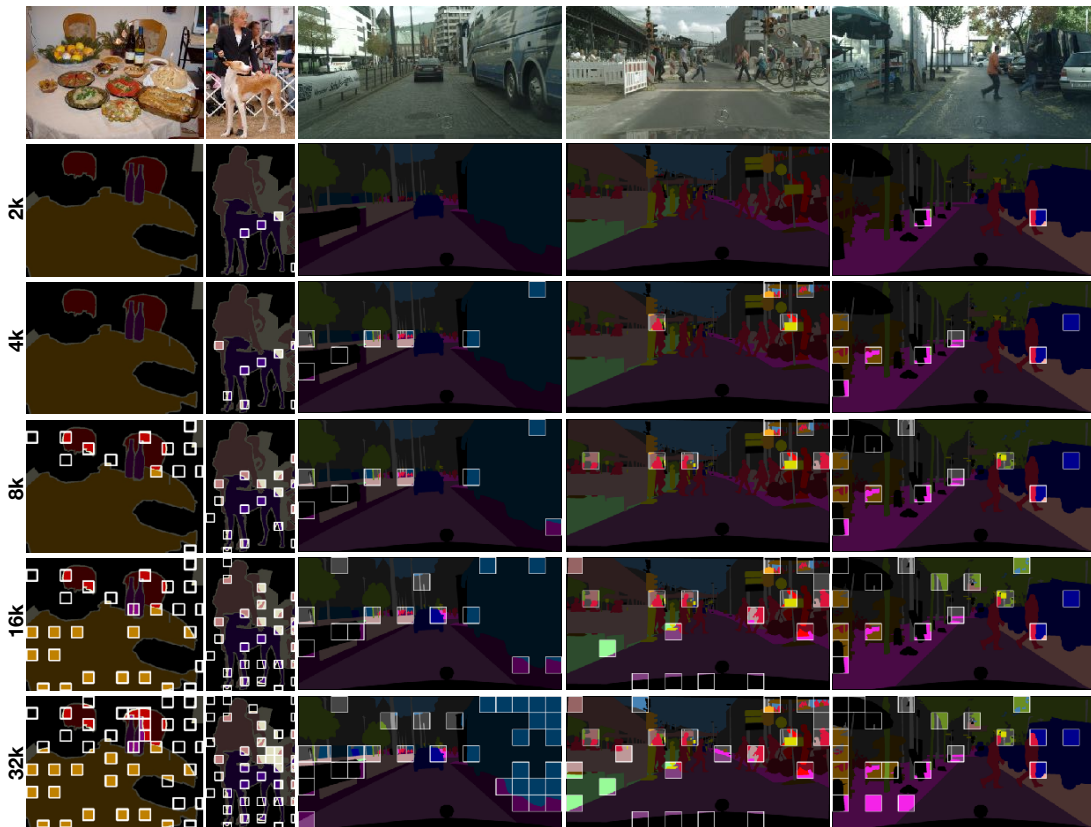
Fig. 4: Visualization of selected regions of Entropy+Spatial with different annotation budgets. Note how our method allows the selection of regions that are neighbors of previously selected regions with increasing annotation budgets.
