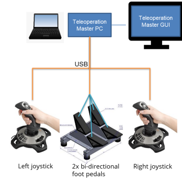
(a) Remote station control
