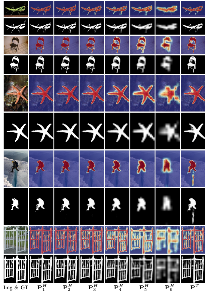
Fig. 4. Feature visualization maps and saliency maps of various intermediate side-outputs of ABiU-Net. Note that \mathbf{P}_1^H is the final output saliency map.
