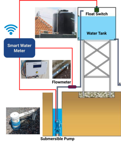
Fig. 4. Installation of Smart Water Meter.
