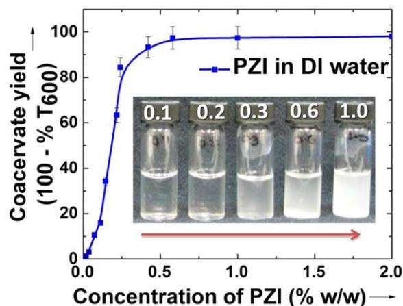
Figure 2. Transmittance with varying concentration of PZI (inset: formation of coacervates at different PZI (% w/w) concentrations. [Color figure can be viewed at wileyonlinelibrary.com]
