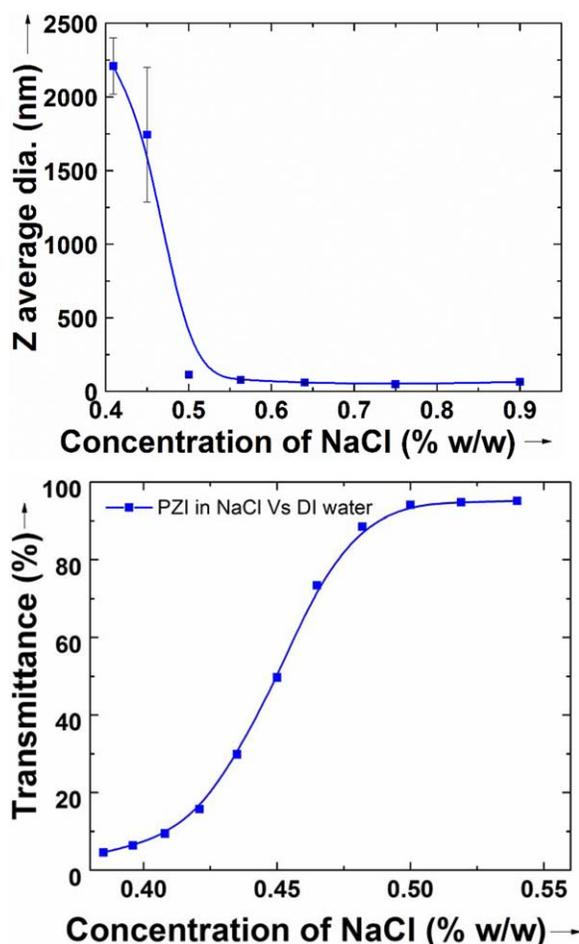
**Figure 7.** Effect of salt concentration on coacervate assembly as determined by DLS (a) and transmittance (b) studies. [Color figure can be viewed at [wileyonlinelibrary.com](http://wileyonlinelibrary.com)]
