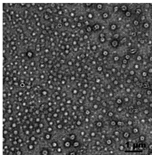
**Figure 6.** TEM micrographs of PZI coacervates in DI water (0.6% w/w) (scale bar: 1  $\mu\text{m}$ ).
