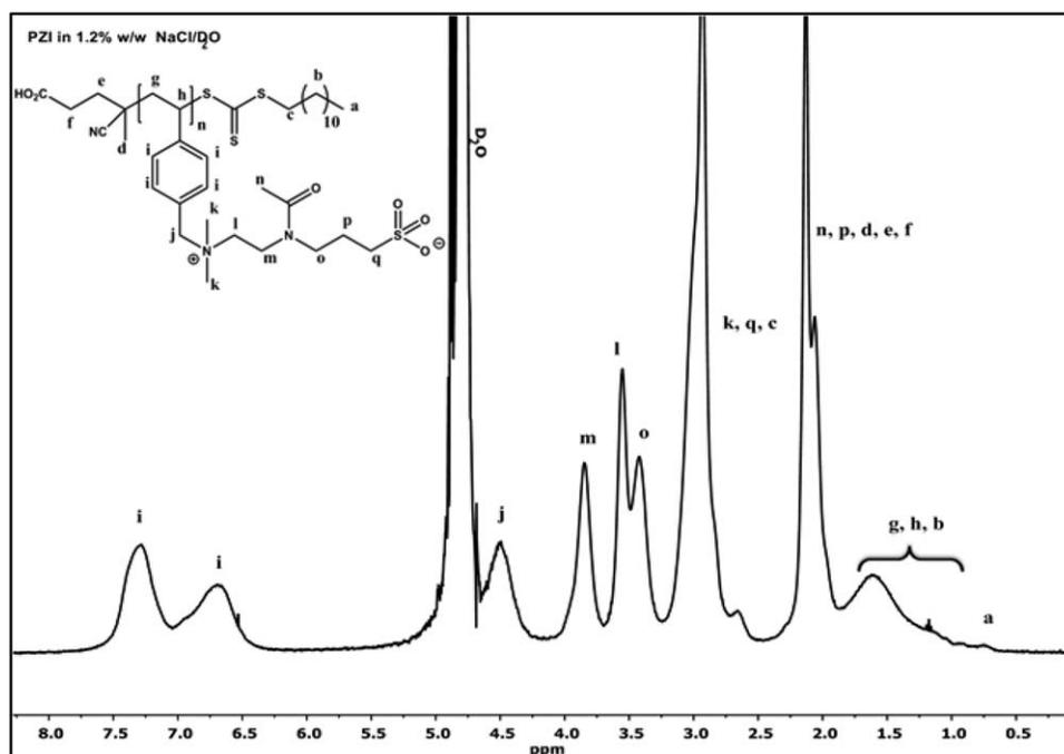
Figure 1.  $^1\text{H}$  NMR of zwitterionic polymer PZI in  $\text{D}_2\text{O}/\text{NaCl}$ .
