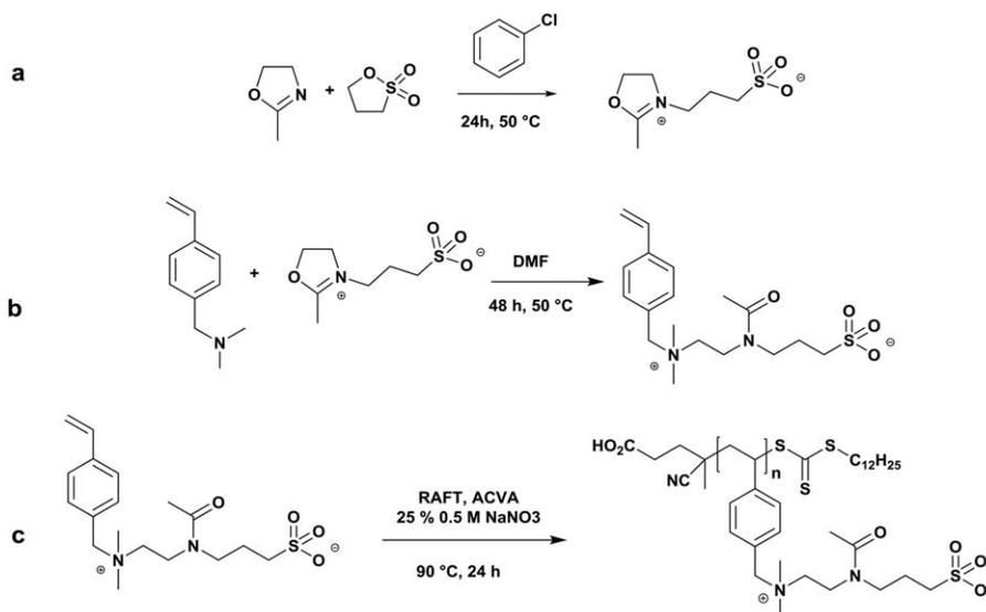
**Scheme 2.** Preparation of (a) zwitterionic adduct,<sup>25,26</sup> (b) zwitterionic monomer, and (c) polymer, PZI.
