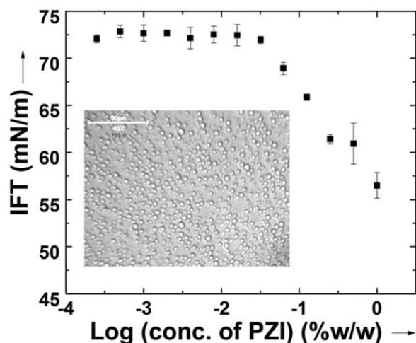
**Figure 3.** Change in interfacial tension with concentration of PZI in DI water (inset: optical microscopic image of 2% w/w PZI coacervates (scale: 50  $\mu\text{m}$ )).
