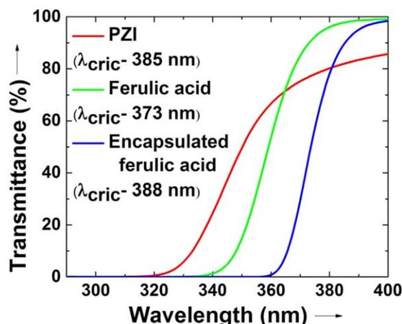
**Figure 9.** Diffused transmittance of PZI, ferulic acid, and the encapsulated coacervate complex. [Color figure can be viewed at [wileyonlinelibrary.com](http://wileyonlinelibrary.com)]
