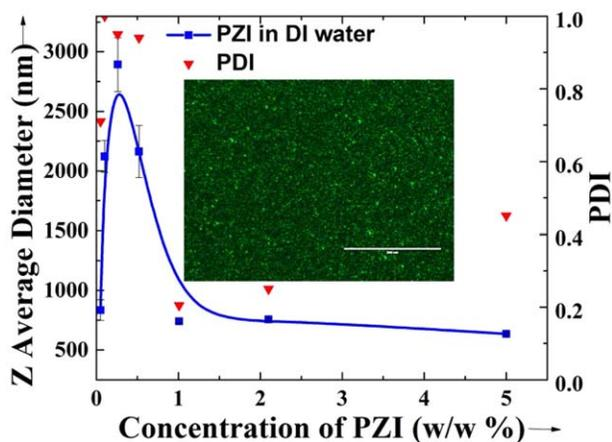
**Figure 4.** Particle size of PZI in DI water at different concentration [inset: PZI (2% w/w) coacervates under fluorescence microscope (scale bar: 200  $\mu\text{m}$ )]. [Color figure can be viewed at wileyonlinelibrary.com]
