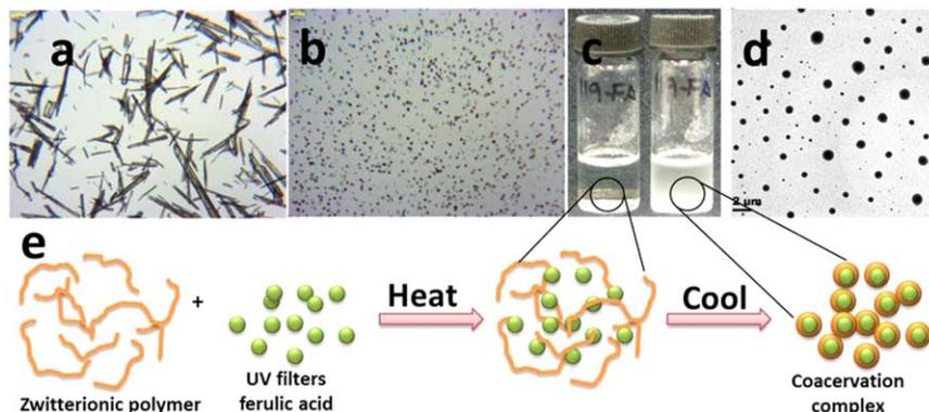
**Figure 8.** Optical microscopy of before (a) and after (b) encapsulation of ferulic acid using PZI (scale bar: 50  $\mu\text{m}$ ); The vials after encapsulation (c) TEM observation of encapsulated ferulic acid dispersed in TFE (scale bar: 2  $\mu\text{m}$ ), (high contrast is due to the high density of ferulic acid (d) and (e) graphic representation of encapsulation through coacervate complex. [Color figure can be viewed at [wileyonlinelibrary.com](http://wileyonlinelibrary.com)]
