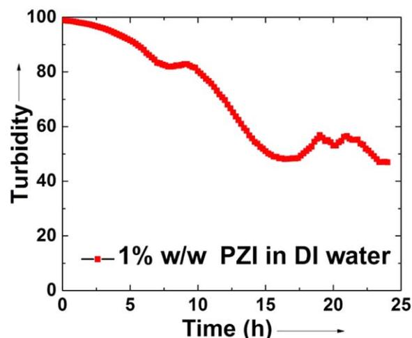
**Figure 5.** Stability of coacervates with time using 1% w/w PZI in DI water. [Color figure can be viewed at wileyonlinelibrary.com]
